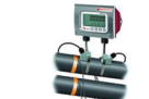
Mobile flow meter to locate leaks -> available on loan from the Watsan Technical Referent
