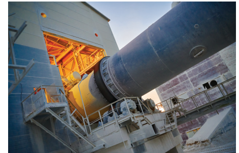
Cement factory rotary furnace at +/- 1450°C
