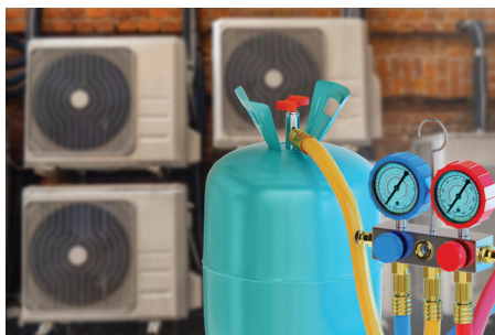
Verification of gas pressure
